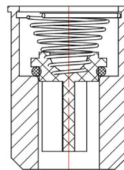
The Termoventiler MV is a mixing valve for mixing tap warm water.
